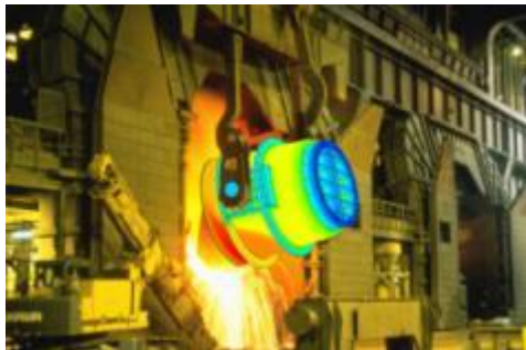
A coupled thermo-structural analysis with software from ANSYS used in developing a new design for a steel-making ladle Courtesy Fundacion ITMA.
