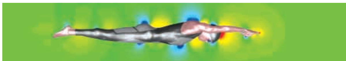
Pressure contours around an elite male swimmer wearing a LZR RACER suit in the glide position
