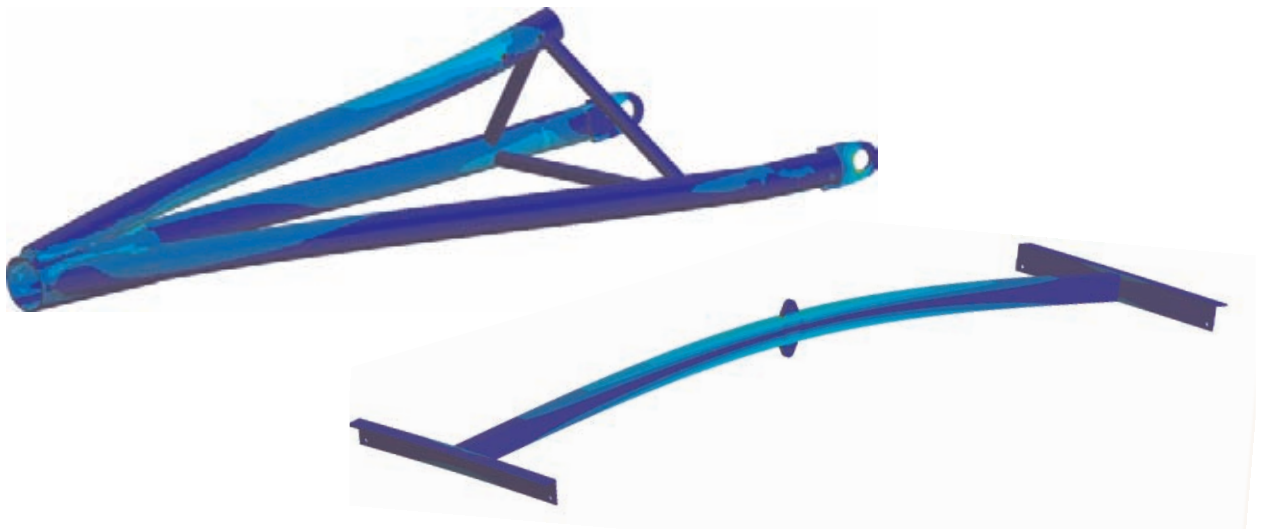
ANSYS DesignSpace structural analysis software was used to determine stress distribution in the Ocean Treader arm (top) and deformation of a spreader beam structure that lifts the machine safely into the water (bottom).
