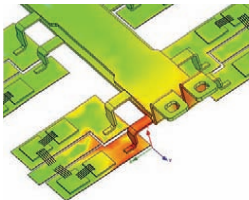
Q3D Extractor model indicates current distribution of an IGBT package.
