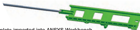
Mast slide plate imported into ANSYS Workbench as a multibody part, which takes advantage of shared topology. The slide plate comprises dozens of individual solids. While these solids may be easily grouped in ANSYS SpaceClaim Direct Modeler to form a single solid, not doing so allows for unique material properties to be assigned to each individual solid.
