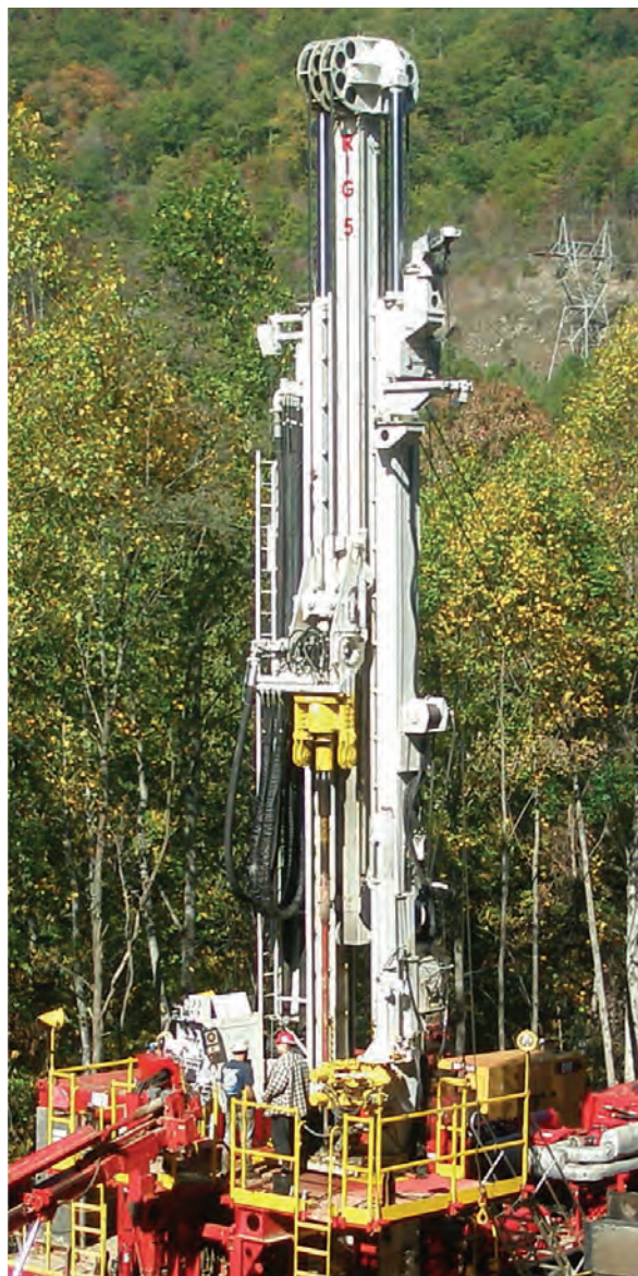
Schramm TXD Rotadrill with mast deployed via extension of its hydraulic cylinder. This equipment is a heavy-hoist, deep-hole, trailer-mounted top-head drive drill rig.
