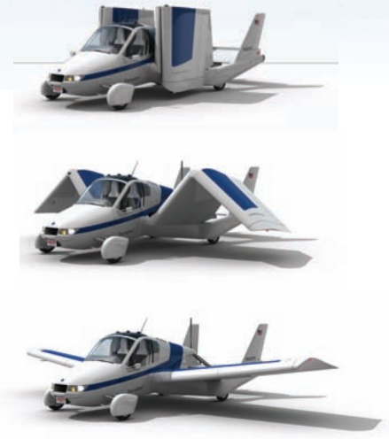
The Transition's foldable wings allow the aircraft to be driven on the highway as well as parked in a typical residential garage.
